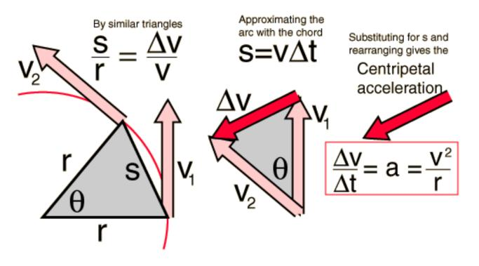
Centripetal means "center seeking" so that means that the acceleration points towards the CENTER of the circle
