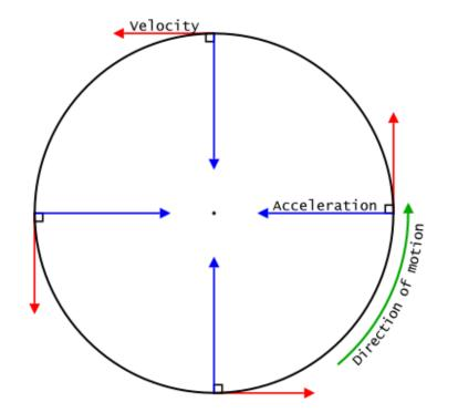
So for an object traveling in a counter-clockwise path. The velocity would be drawn TANGENT to the circle and the acceleration would be drawn TOWARDS the CENTER.
