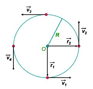
Speed is the MAGNITUDE of the velocity. And while the speed may be constant, the VELOCITY is NOT. Since velocity is a vector with BOTH magnitude AND direction, we see that the direction of the velocity is ALWAYS changing.
