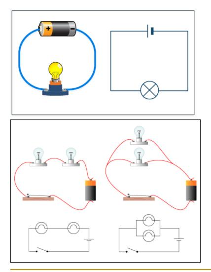
When you are drawing a circuit it may be a wise thing to start by drawing the battery first, then follow along the loop (closed) starting with positive and drawing what you see.
