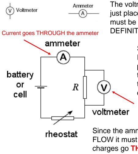
The voltmeter and ammeter cannot be just placed anywhere in the circuit. They must be used according to their DEFINITION.
