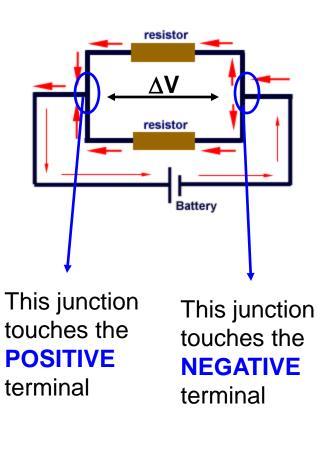
Notice that the JUNCTIONS both touch the POSTIVE and NEGATIVE terminals of the battery. That means you have the SAME potential difference down EACH individual branch of the parallel circuit. This means that the individual voltages drops are equal.
