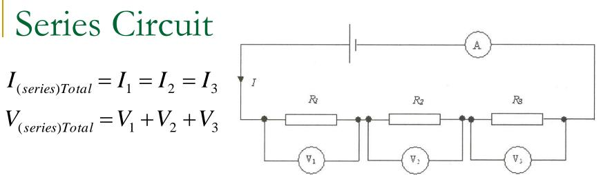
As the current goes through the circuit, the charges must USE ENERGY to get through the resistor. So each individual resistor will get its own individual potential voltage). We call this VOLTAGE DROP.
