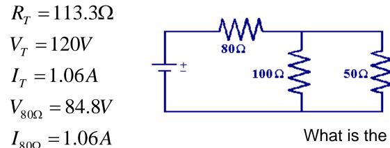
What is the VOLTAGE DROP across the 100 $\Omega$  and 50 $\Omega$  resistor?
