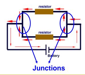
The current going IN to a junction will always equal the current going OUT of a junction.
