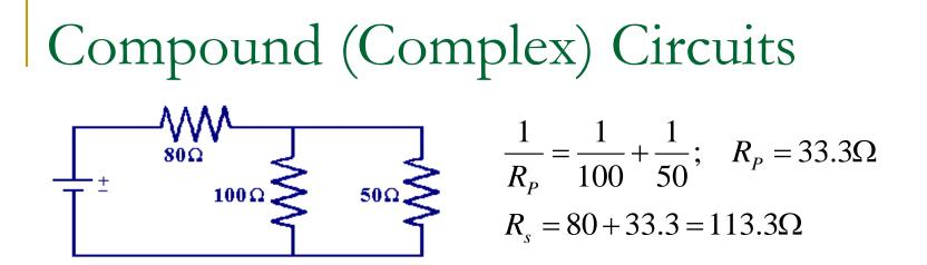
Suppose the potential difference (voltage) is equal to **120V**. What is the total current?
