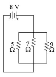
To the left is an example of a parallel circuit. a) What is the total resistance?
