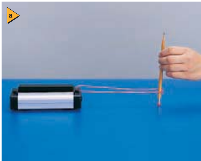
■ Figure 4-3 Because the rubber band is stretched a constant amount, it applies a constant force on the cart, which is designed to be low-friction (a) . The cart's motion can be graphed and shown to be a linear relationship (b) .
