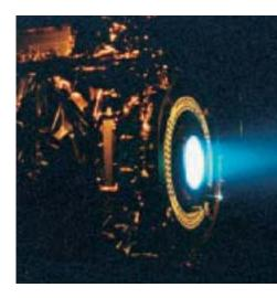
**Figure 9-9** The xenon atoms in the ion engine are ionized by bombarding them with electrons. Then, the positively charged xenon ions are accelerated to high speeds.
