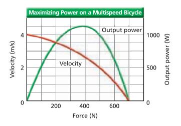
**Figure 10-8** When riding a multispeed bicycle, if the muscles in your body exert a force of 400 N and the speed is 2.6 m/s, the power output is over 1000 W.
