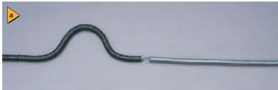
■ Figure 14-11 The junction of the two springs is a boundary between two media. A pulse reaching the boundary ( a ) is partially reflected and partially transmitted ( b ).
