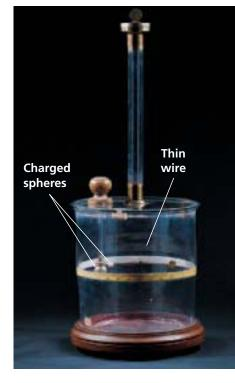
**Figure 20-10** Coulomb used a similar type of apparatus to measure the force between two spheres, A and B. He observed the deflection of A while varying the distance between A and B.
