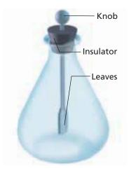
**Figure 20-6** An electroscope is a device used for detecting charges. In a neutral electroscope, the leaves hang loosely, almost touching one another.
