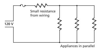
Figure 23-11 The small resistance inherent in wires is in series with the parallel resistances of household appliances.
