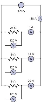
Figure 23-7 In a parallel circuit, the total current is equal to the sum of the currents in the individual paths.
