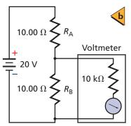
■ Figure 23-12 An ammeter is connected in series with two resistors (a). The small resistance of the ammeter slightly alters the current in the circuit. A voltmeter is connected in parallel with a resistor (b). The high resistance of the voltmeter results in a negligible change in the circuit current and voltage.
