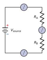
■ Figure 23-3 The ammeters show that the current is the same everywhere in a series circuit.
