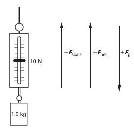
**10.** The 1.0-kg mass and spring scale are being lifted so that the 1.0-kg mass is being accelerated in the positive upward direction at 1.0 m/s<sup>2</sup>. What is the net force acting on the mass?
