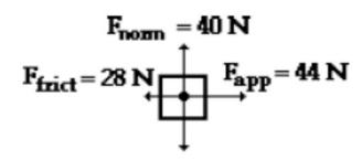
$F_{\text{grav}} = 40 \text{ N}$   $\Sigma F = 16 \text{ N} \qquad \text{right}$  m = 4 kg  $a = 4 \text{ m/s}^2 \qquad \text{right}$
