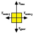
The shipment of the new physics supplies have arrived. They are placed on the freight elevator and transported up to the third floor for delivery to the physics rooms. The free body diagram at the right depicts the forces acting upon the freight elevator as it begins its ascent through the elevator shaft. Use force values to determine the net force, the mass and the acceleration of the elevator. The values of the individual forces are:
