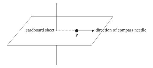
A current is passed through the wire and the compass needle now points in a direction that makes an angle of  $30^{\circ}$  to its original direction as shown below.
