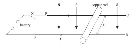
The length of the copper rod between the rails is L. The mass of the copper rod is M. Friction between the copper rod and the rails is negligible.
