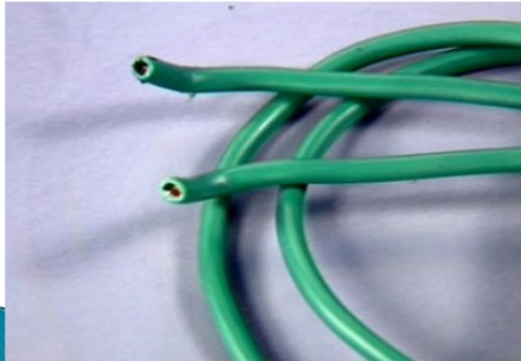
Conductor = Copper Wire Insulator = Plastic sheath
