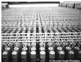
A cascade of centrifuges used for enriching uranium
