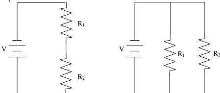
In a series arrangement the resistors are connected end-to-end, such that the charges moving in the loop must pass through all of the resistors. If the resistors are connected in parallel the charges have a "choice" as to which resistor they will pass through. Each charge can pass through only one of the resistors before returning to the voltage source.
