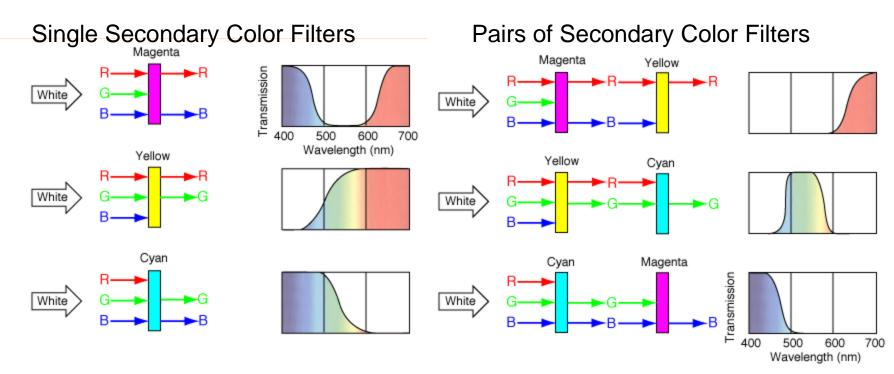
Filters (or pigments) <u>transmit</u> colors that make up the filter color and absorb the others Filters <u>remove</u> their respective complementary color from white light
