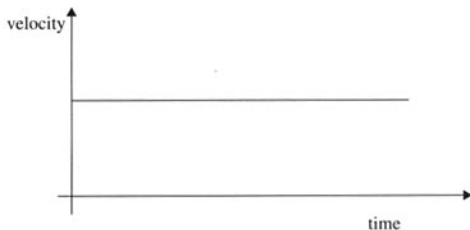
Figure 1.6 Uniform velocity means that the velocity-time graph is a horizontal straight line.
