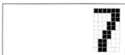
Figure 9.14 The number 7 on a calculator LCD is formed from dark pixels to which a voltage has been applied. The rest of the pixels are bright.
