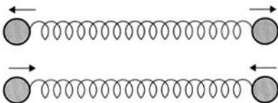
Figure 2.8 The atoms of a diatomic molecule vibrate. The energy associated with the vibration is quantized.
