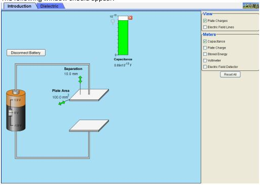
Using the default separation and plate area, adjust the battery between -1.5 V and 1.5 V. Write down your observations.
